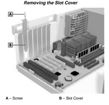
Save the screw for installing the expansion board. Be sure to save the slot cover for future use.
